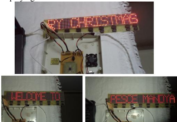
Fig. 6 Dot-matrix display before updating (top) and after updating (below)
